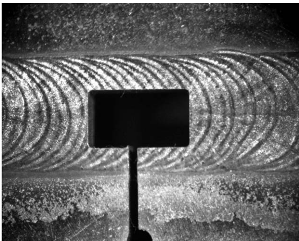
Fig. 1. Top view of 316LN welded part and the specimen cutting configuration. The picture shows the welded joint produced by DIN1.4455 filler and the dimension of the rectangular cut is 3.95 mm \times 2.85 mm.
